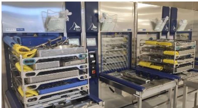
Figure 5: Automated washing with pass-through equipment that brings the instruments to packaging area
